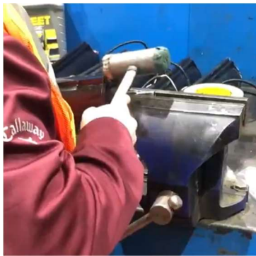
Figure 2: Rubber Mallet Use To Release Dust Cover
