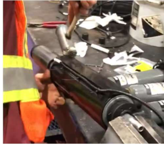
Figure 4: Using Rubber Mallet To Seat Dust Cover on Retaining Ring.
