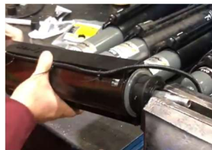
Figure 3: Install Dust Cover & Center Over Grey Retaining Ring.
