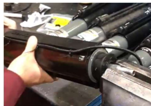
Figure 2: Install Dust Cover & Center Over Grey Retaining Ring.
