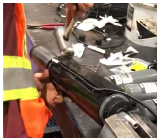
Figure 3: Using Rubber Mallet To Seat Dust Cover on Retaining Ring.
