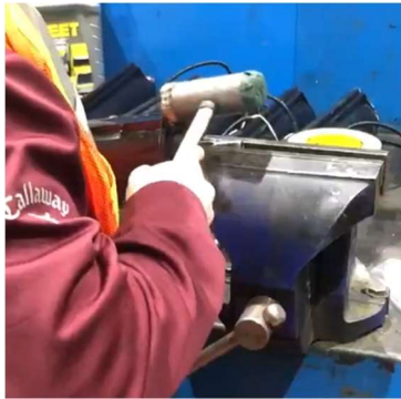
Figure 1: Rubbet Mallet Use to Release Dust Cover
