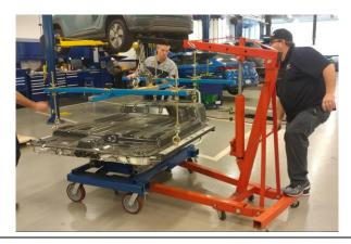
Move the EV battery from the vehicle to the shipping crate and carefully lower it in place so it is centered on the crate.
