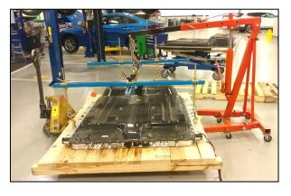
g) Transfer the Lifting Fixture Kit back to install on the replacement battery. Raise the replacement battery from its temporary resting point and place it onto the
