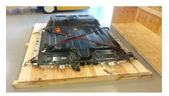
J-2. For Kona EV and 2020MY~ Ioniq EV battery with coolant, ensure there will be no coolant leaking out of the battery onto the shipping crate.
