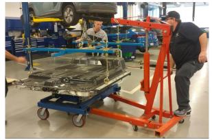
F-3. Install the replacement battery to the vehicle in reverse of the shop manual removal instructions.
