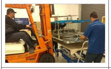
f) Move the EV battery from the vehicle to the shipping crate and carefully lower it in place so it is centered on the crate.
