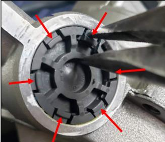
11d-2. Remove the grease plug (K).
