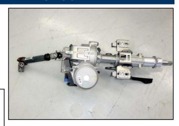
4. Only remove the lower pinch bolt (A) on the steering universal joint assembly to remove the C-MDPS assembly.
