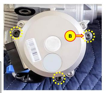
TSB #: 20-ST-003H Page 6 of 14 6. Remove the motor assembly (C).
