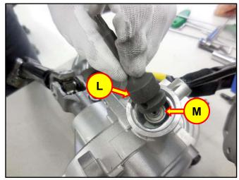
11d-4. Using a plastic hammer or rubber mallet, lightly tap the extension to free the worm shaft assembly.
