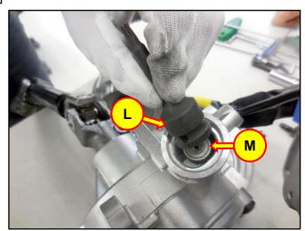
11c-5. Using a plastic hammer or rubber mallet, lightly tap the extension to free the worm shaft assembly.
