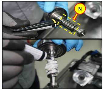
14. Carefully reinstall the new worm shaft assembly.
