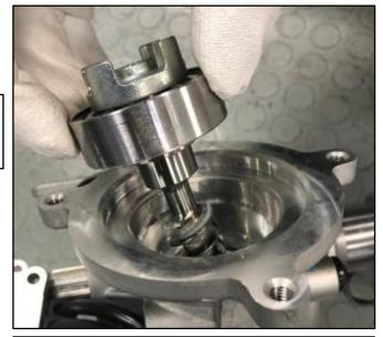
13. Apply the entire contents of the supplied grease evenly onto the new worm gear (N).
