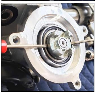
c. If either of the above methods are unsuccessful, move to step 11c (Page 8) for an alternate method of removal.
