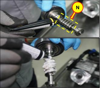
14. Carefully reinstall the new worm shaft assembly.
