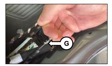
7a. Check the hood release cable coupler is attached properly and that the two cable attachments (black and white ends) are fully inserted into the mounting bracket(s).
