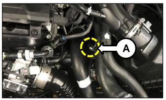
2a. Confirm that the hose clamp (A) break away nut head (B) is not present and that the hose is properly inserted/seated. If so, this action is complete.
