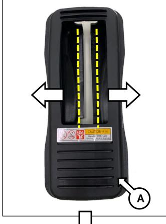
2. Insert the ICCB device (B) into the protection cover (A) as shown.
