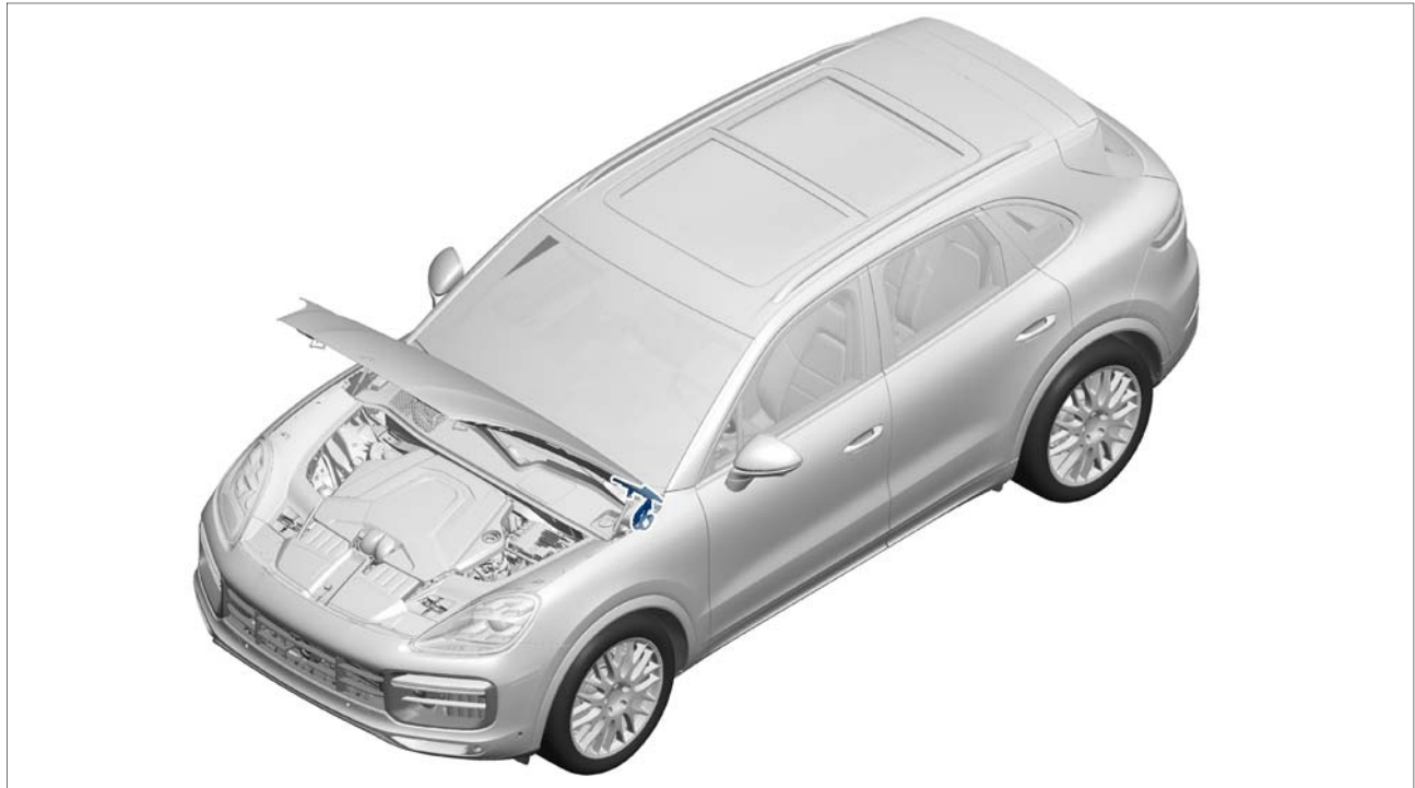
Installation position of front lid hinge
