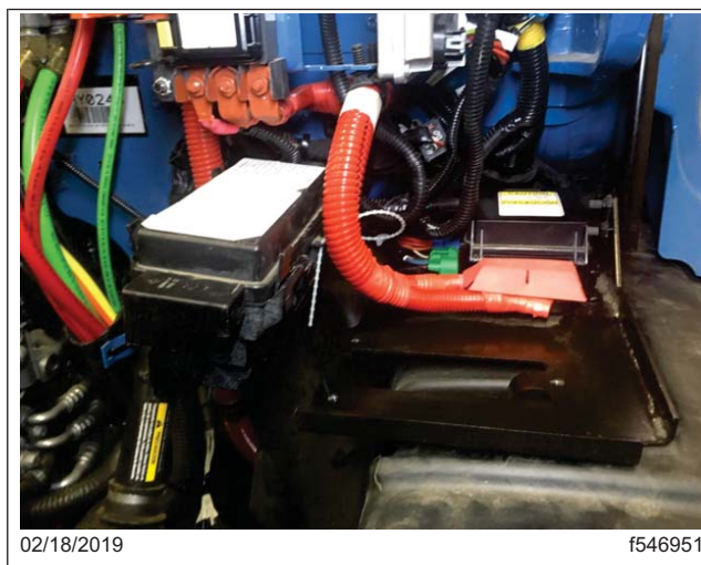
Fig. 6, Quarter Fender and Powertrain Power Distribution Module (PTPDM) Installed on the Vehicle
