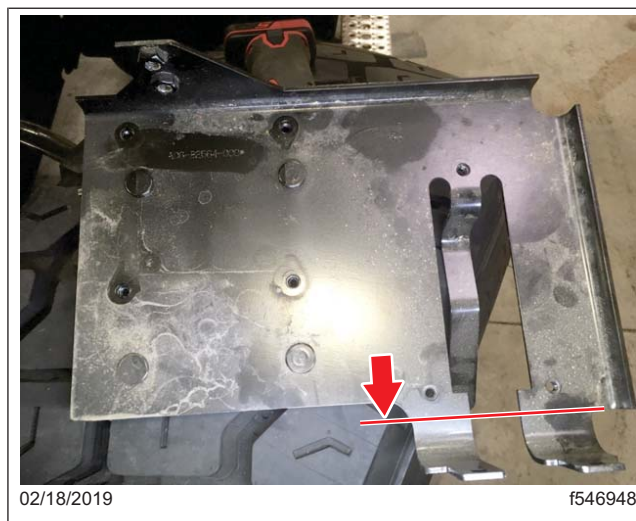
Fig. 2, Cutting the Powertrain Power Distribution Module (PTPDM) Bracket Mounting Tabs
