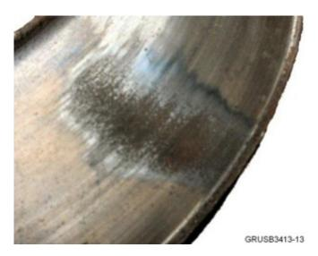
Discoloration and/or visible hard spots indicate brakes that have overheated.
