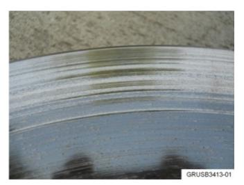
Grooves are formed when debris is trapped between the pad and the disc. Debris entry is inherent in the disc brake cooling design.
