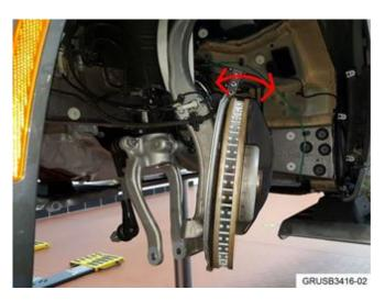
Brake disc thickness variation is the result of lateral runout in the face of the brake disc.
