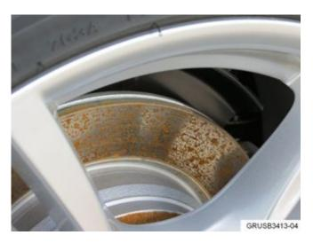
Brake disc friction surfaces consist of exposed metal. When not in use and exposed to environmental elements (moisture, salt, dirt), surface rust can form. During initial braking, this will self-clean and an audible groan and/or noise is temporarily heard until the disc surface is cleaned.
