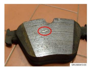
Improper "bedding in" of the new brake pads and discs can cause the rotor material to flake off. This debris can become lodged in the pads and cause this appearance.
