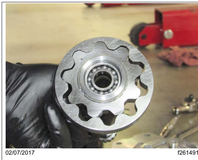
Fig. 11, Oil Pump and Drive Shaft
