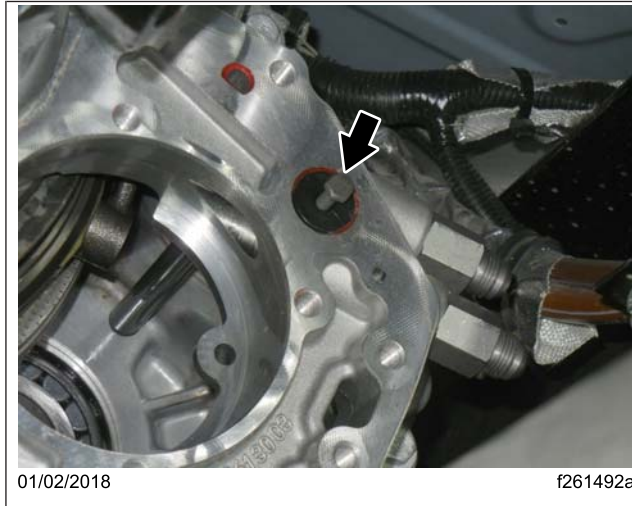
Fig. 10, Original Control Valve
