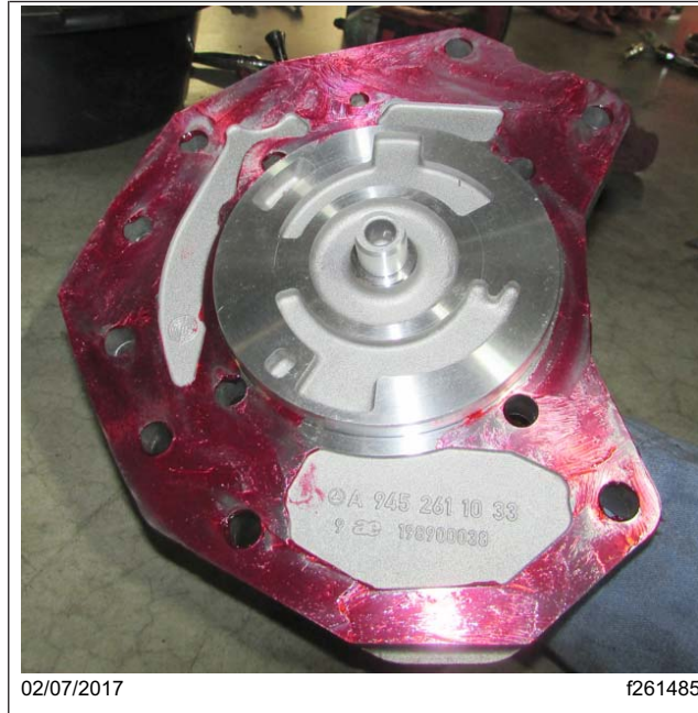
Fig. 12, Sealant Applied to Pump Cover
