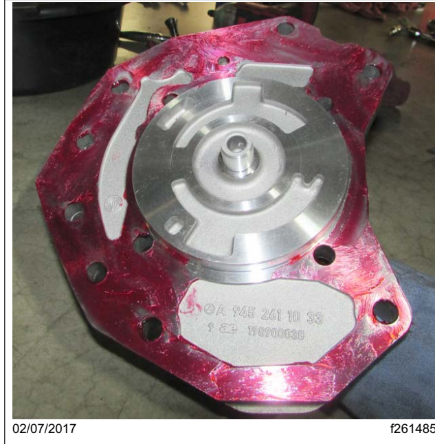
Fig. 12, Sealant Applied to Pump Cover
