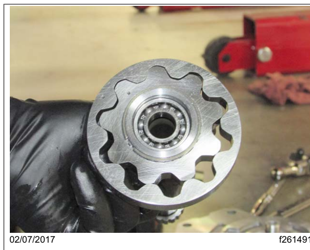
Fig. 11, Oil Pump and Drive Shaft
