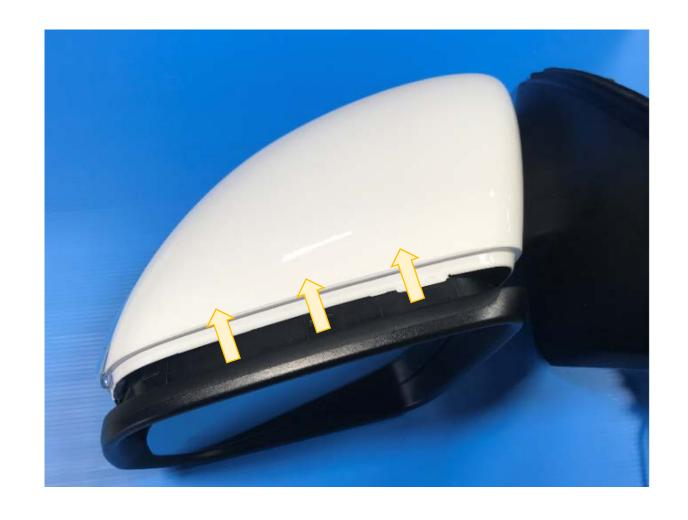
2. Remove paint on the bottom of the tongue area on the housing cover.
