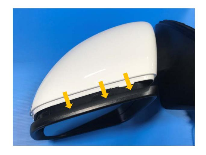
4. Verify tape can not be seen in the gap between the bezel and the housing cover.
