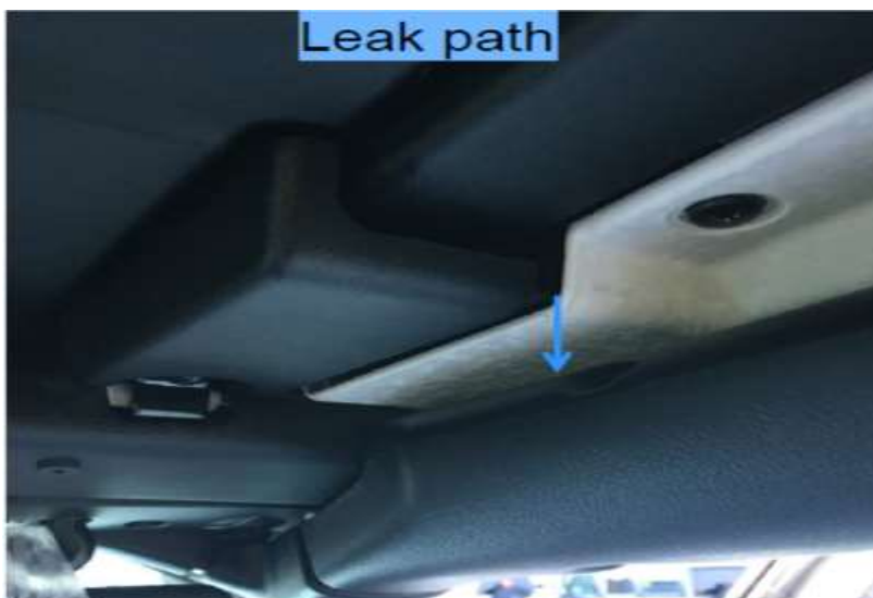
Fig 1 water leak path
