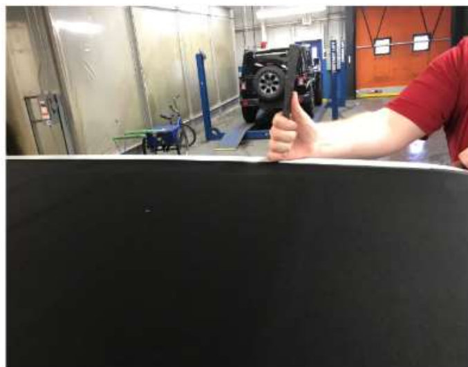
Fig 2 applying pressure to wet out (bed) the butyl.
