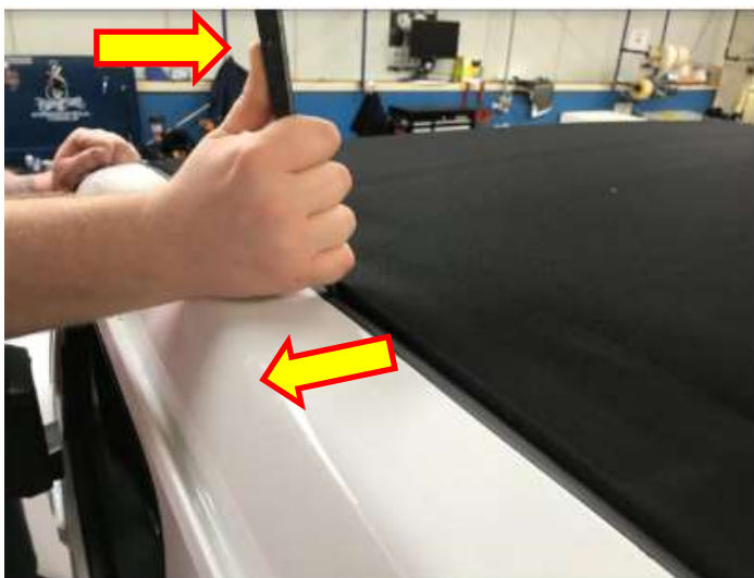
Fig 2 applying pressure to wet out (bed) the butyl.
