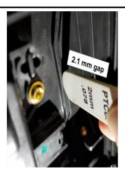
**Repair Procedure:** If determined that there is a gap present causing the whistle noise the replacement of the HVAC box assembly is required.
