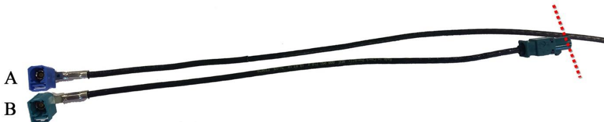
Figure 2. Measure the cut point on the vehicle's antenna coaxial wiring (A) based on the length of the replacement coaxial "Adapter Antenna Cable" (B). The removed length of cable from A should be equal to the length of cable B.
