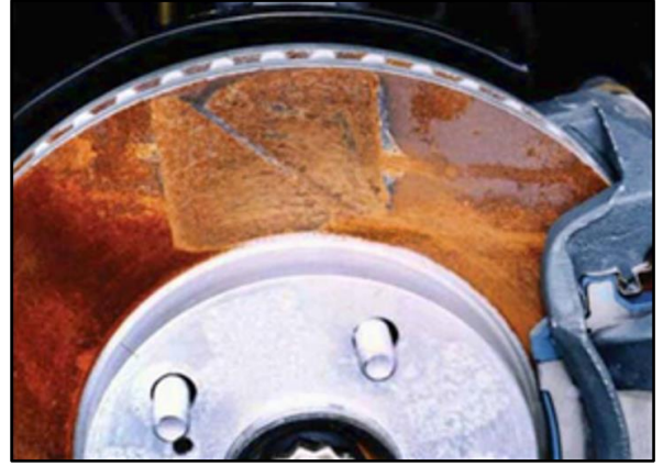
Figure 2. Severe Rust on Rotor (Hard to Remove by Braking)
