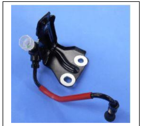
Figure 19. Brake Actuator Tube No. 3 and Brake Actuator Way in the Form of Assembly
