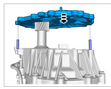
Caution! Make sure that the component is correctly located on the locating dowels.
