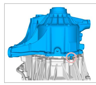
Caution! Make sure that the component is correctly located on the locating dowels.
