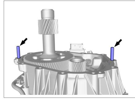
Note! As an alternative if a tool is not at hand, use two bolts M8 x 60 mm with heads cut off.
