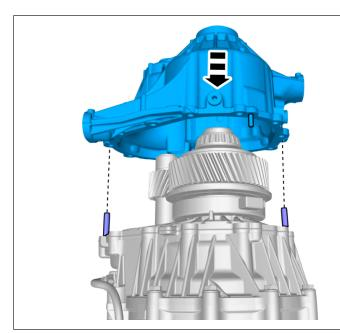
Caution! Make sure that the component is correctly located on the locating dowels.
