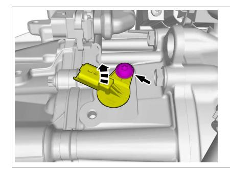
Remove the screw. Lift the marked component up
