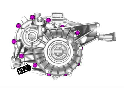
Note! Make sure that locating studs remains in the timing gear casing.
