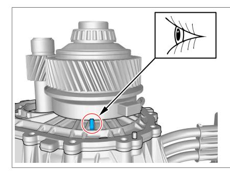
Note! Make sure that the installation marks are aligned.
