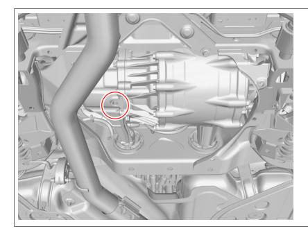
Caution! The fluid must be allowed to escape until a continuous flow changes into single drops.
