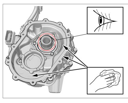
Note! Check the component. if any damage is shown, the whole complete ERAD is to be exchanged.
