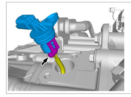
Disconnect the connector. Remove the marked part.
