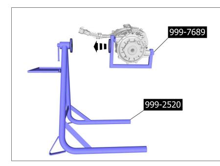
Special Tool: T9992520, FLOOR STAND (TO FIXTURES) - Substitute with an appropriate stand as necessary
