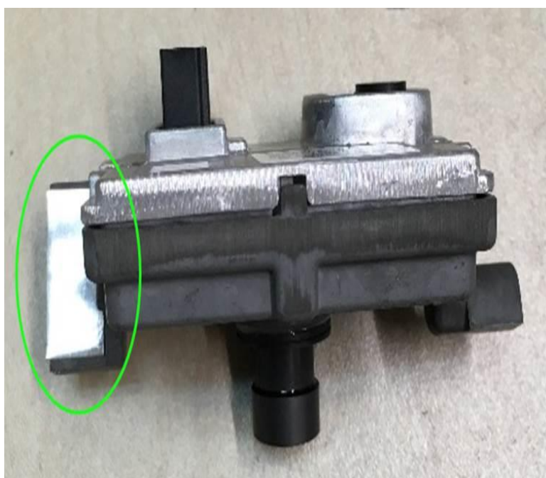
Figure 1. How to correctly attach the aluminum adhesive foil on the front camera for assistance systems -R242-.
