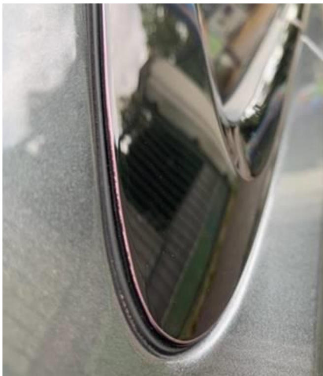
Figure 3. Discolored black optic trim around rear side window.
