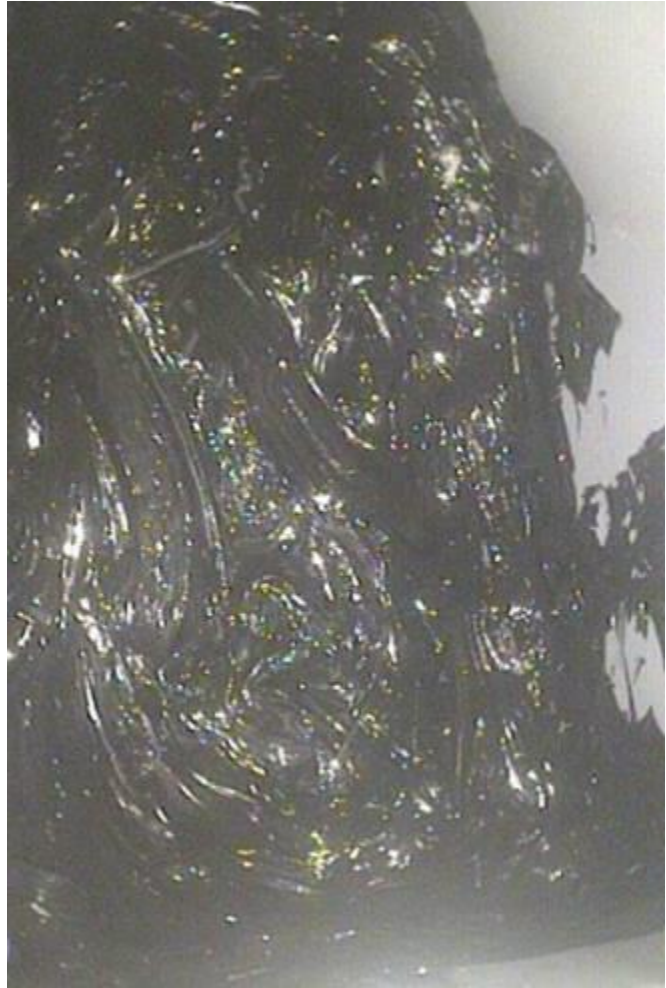
Figure 13. Sealer completely applied and distributed.
