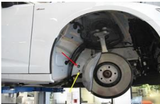
Figure 5. Point of entry for the borescope.
