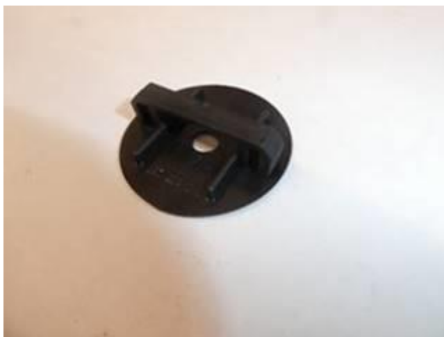
Figure 15. New longitudinal member plugs with integrated drain.
