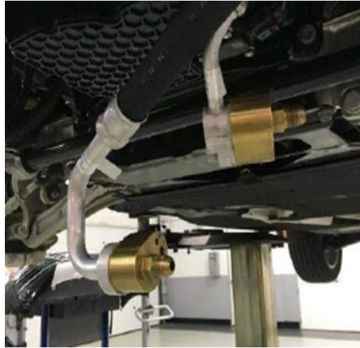
Figure 6. Installation of VAS 6338/3 and 6338/12.
