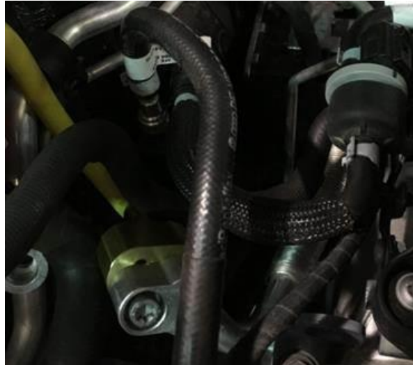
Figure 17. Attaching service station and flush hoses to rear A/C lines.
