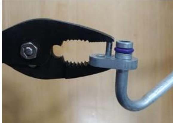
Figure 16. Installation of rear refrigerant line dowel pin.
