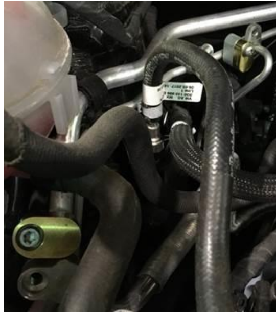
Figure 4b. Installation of Low side rear A/C Line connection block adaptor VAS 6338/5
