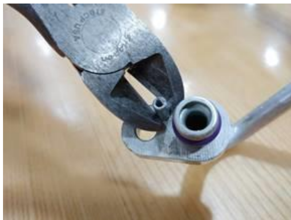
Figure 15. Removal of dowel pin.
