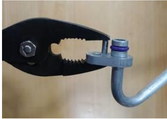
Figure 16. Installation of rear refrigerant line dowel pin.
