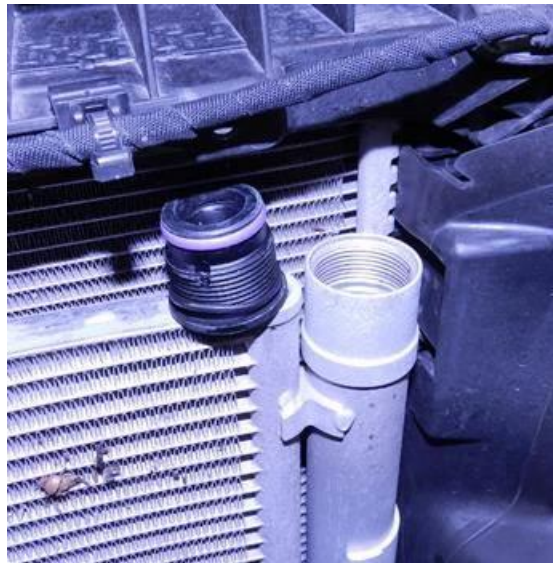
Figure 2. Location of the Receiver Drier
