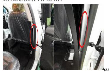
Using an appropriate trim tool, partially remove the center pillar lower trim panel to gain access to the body inner panel as shown. Refer to Center Pillar Lower Trim Panel Replacement in SI.
