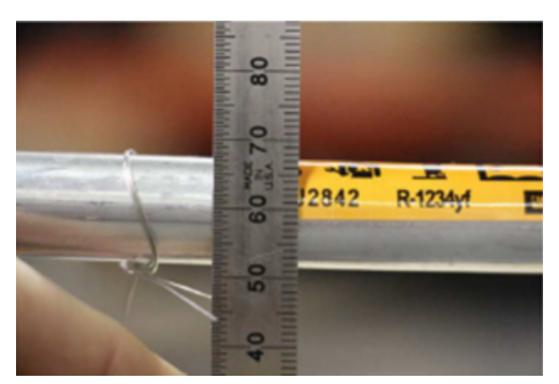
If the TXV tubes are bent down do not attempt to adjust the tubes to allow installation of the evaporator in the HVAC case. If the tubes are bent or adjusted back into position this will result in a slow leak from the lock ring joint.
