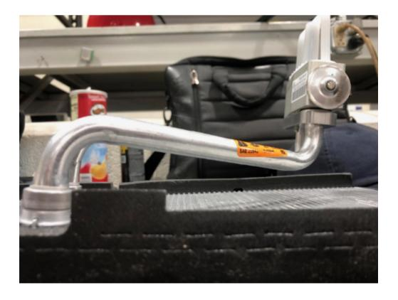
There should be a distance of 50-60 mm. when measuring from the core to the center of the TXV tubes as shown below.
