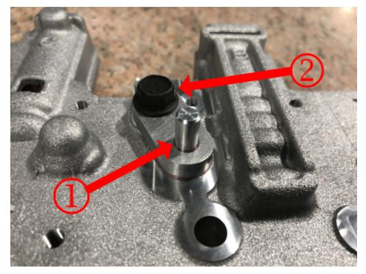
If the plug and retaining bolt are missing as shown in the picture below please fill out the WPC part request form and send it to the WPC following the instructions below.
