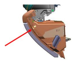
2) Push right hand Rod in-board. This will un-latch the Glove Box Door and open it.
