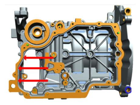
The 4 mm (0.16 in) bead of sealant must be centered on / follow this grove on the Lower Crankcase Extension.
