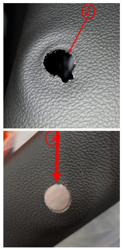
Install a new door panel lock rod bezel ring on the affected door. Bezels are available from CCA, see the "Parts Information" section below. Do not repair any unaffected doors.
