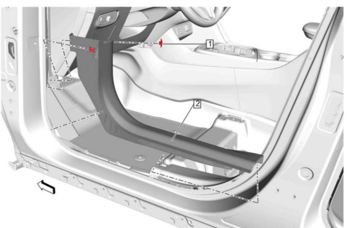
Reinstall the left front side door sill garnish molding (2). Refer to Front Side Door Sill Garnish Molding Replacement in SI.
