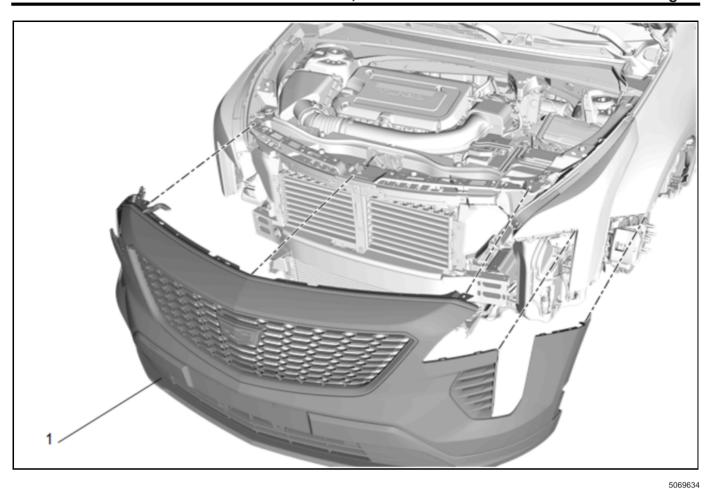
6. Reinstall the front fascia (1). Refer to *Front Bumper Fascia Removal and Installation* in SI.
