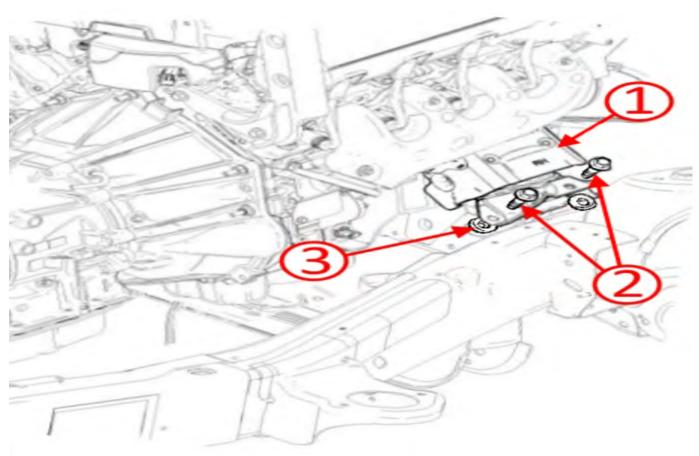
**Note:** Pause after loosening any of the mount bolts during these steps to determine the effect of the idle vibration on the Pico, at the seat track while making note of effect from each bolt location.
