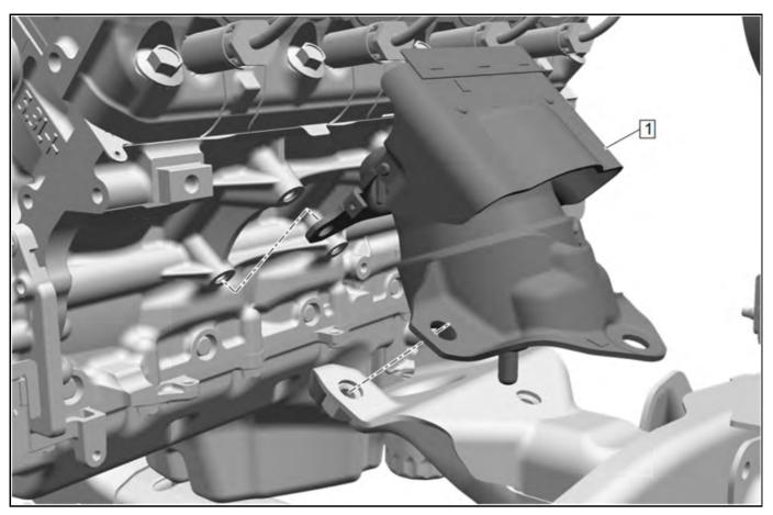
**Note:** Initial removal of the engine mounts will require the removal of the exhaust manifolds.
