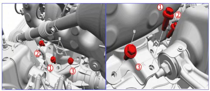
**Important:** Do Not use Impact wrenches when tightening the engine mount to frame bolts, or damage to threads in the frame may result.
