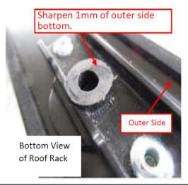
Sharpen bottom of spacer diagonally (sharpening amounts: inner = 0 mm - outer = 1mm)
