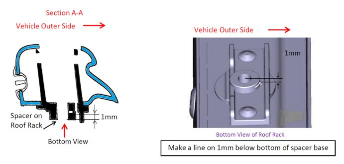
B. Sharpen the bottom of spacer with sandpaper referring to the line which you made in the previous step (A).
