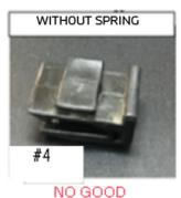
The Clip may be broken or deformed and will no longer have resilience or spring action.
