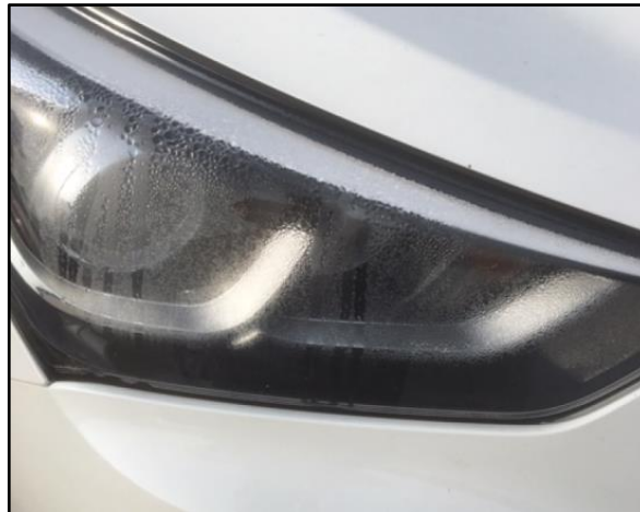
Water collecting inside the headlamp
