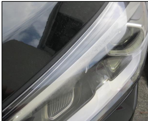
Normal condensation in the headlamp
