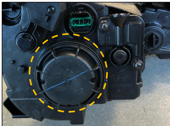
Example of dust cap location
