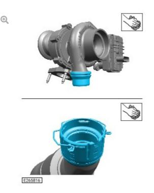
Clean off any oil residue found in and around end of the charge air cooler intake pipe that connects to the turbocharger and the turbocharger outlet, as shown in the illustration.
