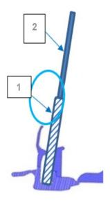
Section view of GLASS RUN-CHANNEL
