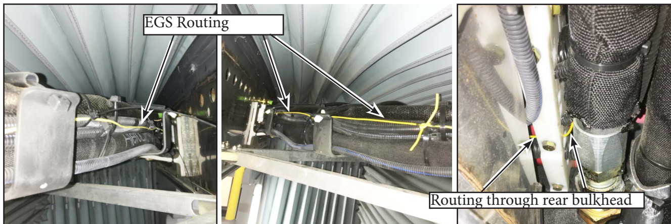
Figure 24 - Front-to-Back Cable Routing in the EGS
