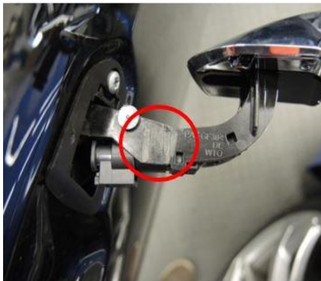
Figure 3. Door handle shown with #1 and #2 ribs removed, leaving an even surface.
