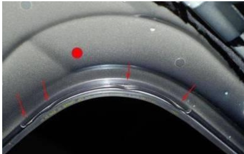
Figure 2. The red dot shows the location of the 10 mm hole to be drilled.
