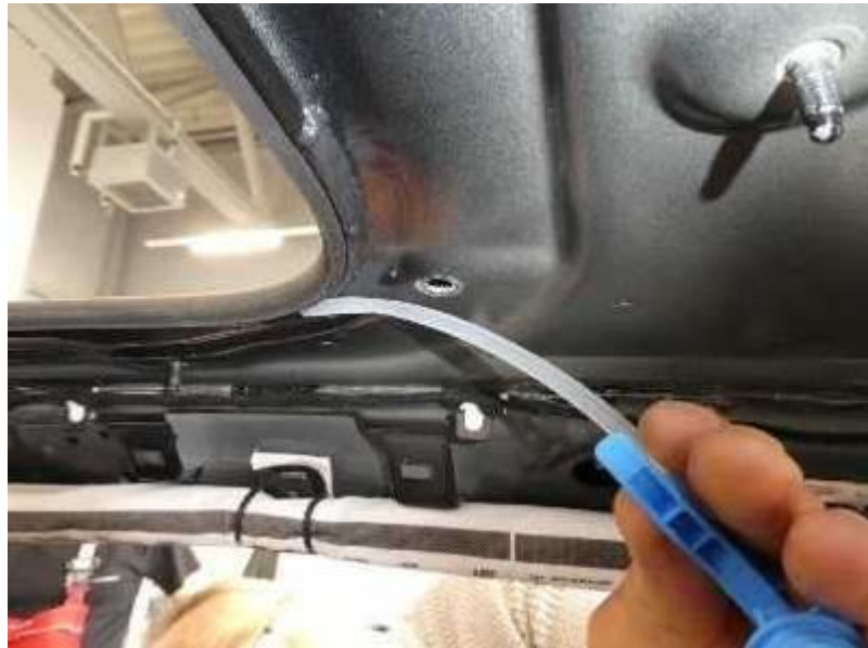
Figure 10. Hose insertion simulation in the 'A' direction.
