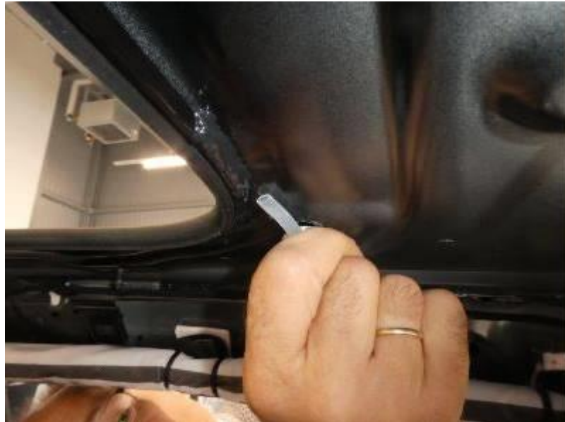
Figure 9. Hose insertion simulation in the 'B' direction.
