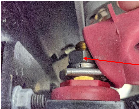
Install the cable using existing hardware
