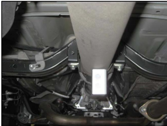
Figure 11. CORRECT Placement of Digital Angle Gauge
