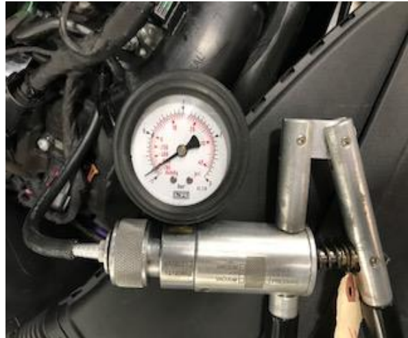
Figure 1. Checking the vacuum at the output port of N649.
