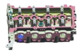
Note: The Cylinder Head part number provided comes assembled with Valves, Springs and Cylinder Head Bolts.
