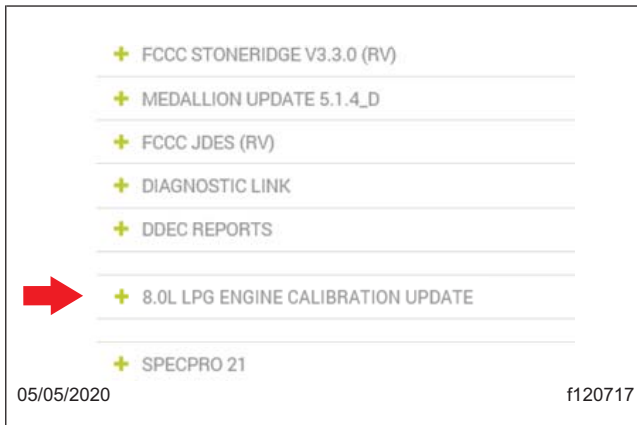
Fig. 2, Selecting 8.0L LPG Engine Calibration Update
