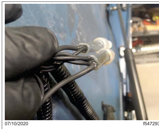
Fig. 5, Wires Sealed with Protective Gel
