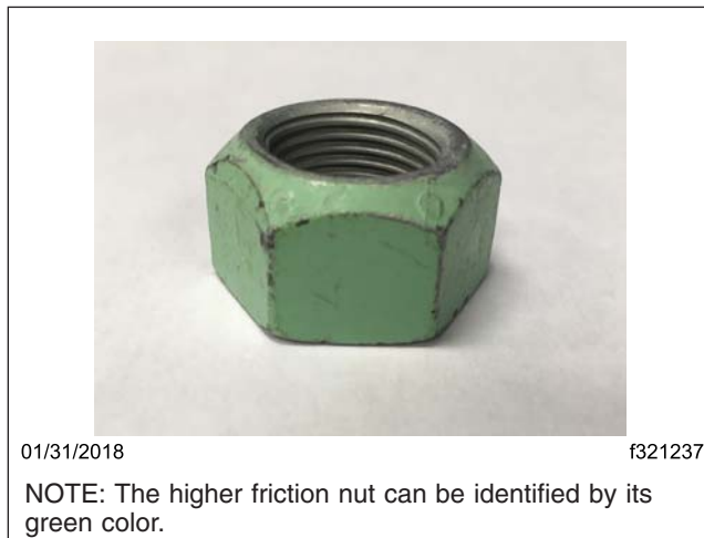
Fig. 1, New High Friction Nut
