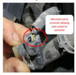
2 – Review Wiring at the Upper Control arm Clip for tight clip, wires underneath the convolute for damage or rubbing
